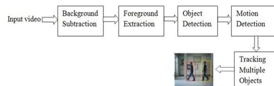
**Figure 1.** General overview of object detection and tracking
